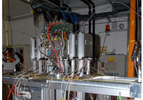
Fig. 56: Photograph of the testbeam setup of the combined pixel - strip testbeam in November 2010. The testbeam was held at the Jessica site of the COSY storage ring in Jülich. In this picture the beam is coming from the left side, flying through two layers of strip detectors, four layers of pixel detectors and at the end again through two layers of strip detectors.
