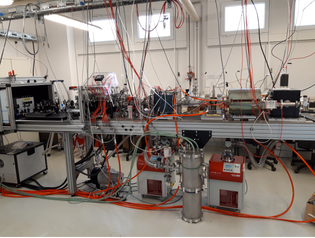
Fig. 1: The experimental setup (from left to right): The Nd:YAG laser inside a shielding box, laser optics, interaction chamber with pulsed nozzle, ionizer, and the components of the Lamb-shift polarimeter.
