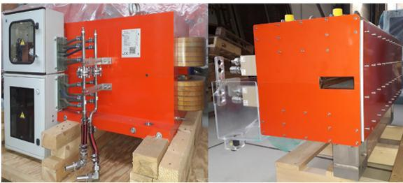
Figure 36: Left: Injection dipole magnet with electrical and cooling water connections, deflection angle  $7^\circ$ . Right: Injection septum with screen on the right hand side for shielding the circulating beam. The rectangular opening is for the pipe of the incoming beam. Deflection angle is  $3.817^\circ$  for each of the 2 septa.
