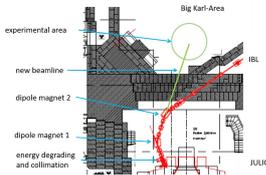
Position of energy degrader and dipole magnet to obtain optimal experimental conditions in Big Karl area with reduced neutron background.
