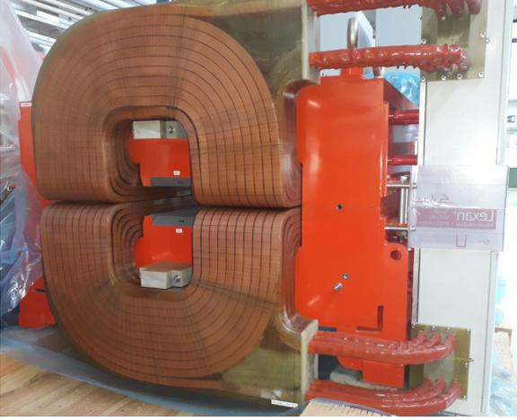
Figure 39: Chicane dipole magnet, connection side
