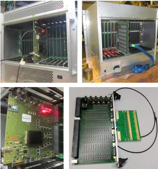
Figure 1: Top: The OpenVPX crate with one ADC processing board and one analog board inserted, (left) front side with processing board, (right) rear side with the preamplifier board and one Samtec 32 channel coaxial cable. Bottom: (left) The ADC board, the central FPGA is visible in the lower half of the board and the ADCs behind. (right) Preamplifier board with an adapter for direct coupling of signals into the preamplifier board.
