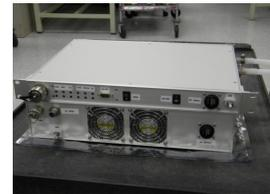
Custom made 100W power amplifiers were crafted by Nanowave Tech Inc. to optimize gain, phase and group delay for best cooling performance
