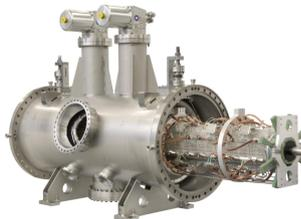
Pick-up for the stochastic cooling system of HESR inside a tank
