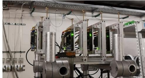
Figure 1: The MuPix8 beam telescope
