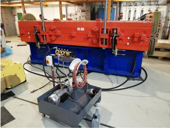
Figure 35: HESR main dipole magnet with accessories for lifting the upper yoke for maintenance purposes. The cycle of lifting and lowering the upper yoke can be watched online<sup>7</sup>.
