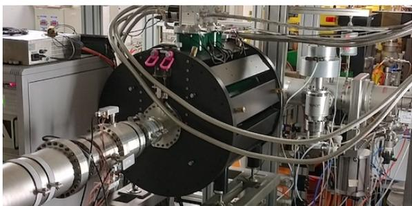
Figure 1: A picture of the Siberian Snake installed in COSY.
