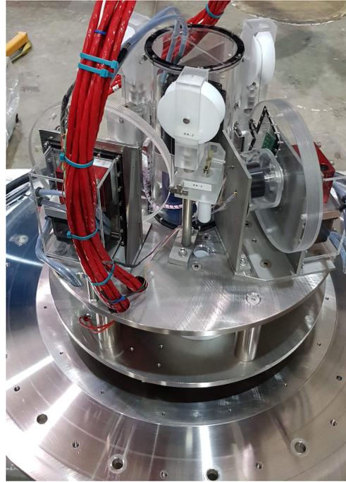
Figure 22: A photograph of the Automated Calibration Unit, which will be used to lower sources into the scintillator volume of OSIRIS detector. The different pulleys allow the automatic selection and use of different pre-mounted calibration sources.
