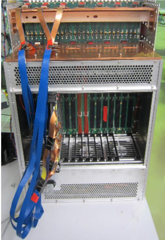
Figure 3: The rear view of the OpenVPX crate with one amplifier board (bottom part) connected with the HV decoupling crate (upper part) with modified SAMTEC cables.
