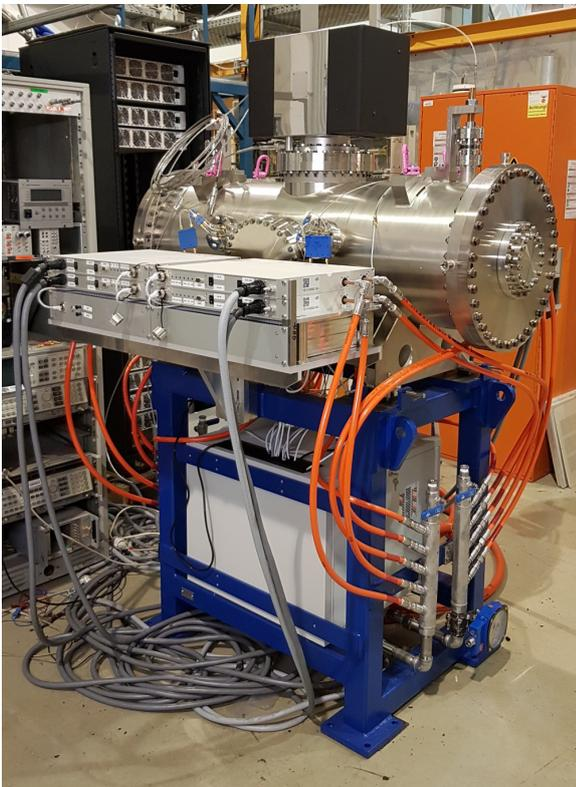
Figure 35: Stochastic kicker tank on girder. One half of the water-cooled high power amplifiers is visible, the other half is on the back.
