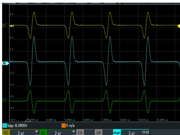
Figure 2: A 20% Barrier-Bucket reaching peak-peak voltage of  $V_{pp} = 8.3$  kV. Yellow: Voltage at the upstream-sided rings of the gap (1:1000), green: Voltage at the downstream-sided rings of the gap (1:1000), blue difference of both.
