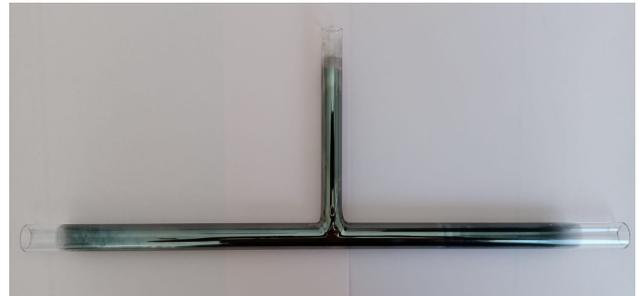
Figure 2: carbon coated storage cell.
