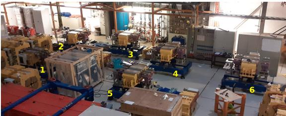
Figure 24: Assembly hall: Benches for quadrupole girders of the arc sections.
