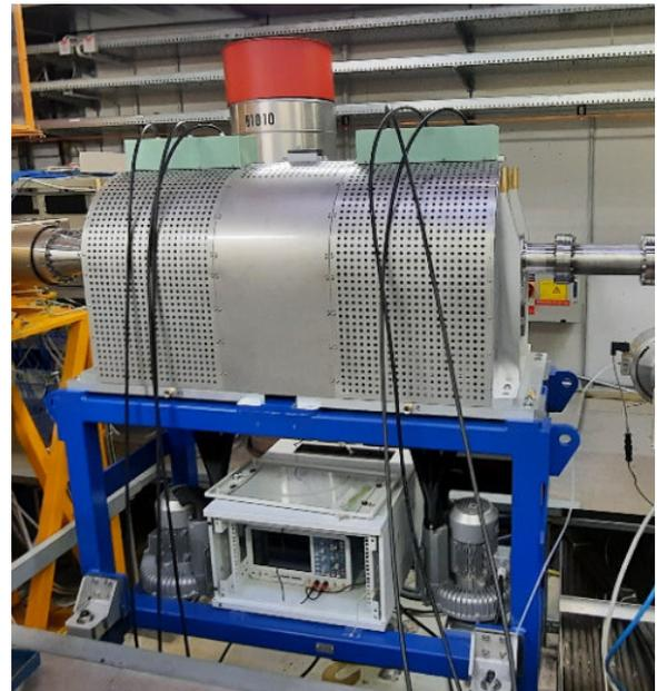
Figure 25: HESR cavity installed in COSY. Note the fans below each resonator.
