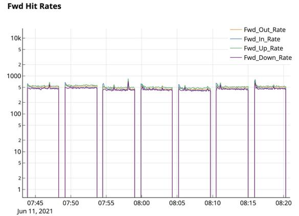
Figure 5: The hit rates on the four scintillator detectors measuring the proton-proton elastic scattering at the beam momentum of  $3.0 \text{ GeV}/c$ , which the beam was running at the centre of the beam pipe and without evident beam halo.
