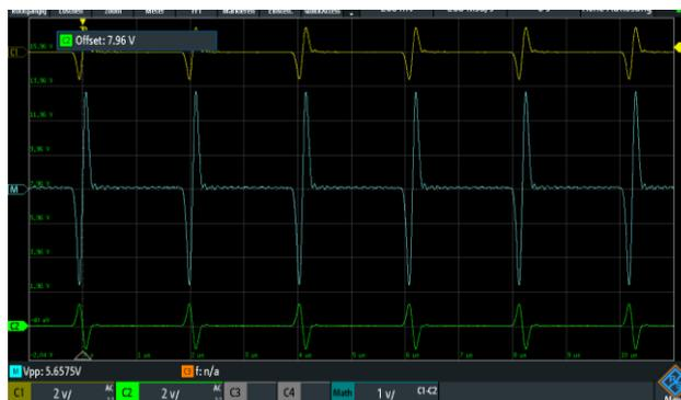
Figure 3: A 10% Barrier-Bucket reaching peak-peak voltage of  $V_{pp} = 5.6$  kV. Yellow: Voltage at the upstream-sided rings of the gap (1:1000), green: Voltage at the downstream-sided rings of the gap (1:1000), blue difference of both.
