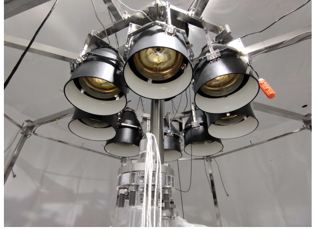
Figure 27: The first eight PMT modules of OSIRIS, which were installed above the acrylic vessel. The PMTs feature magnetic shieldings to reduce electronic noise and signal disturbances caused by the Earth's magnetic field. The white ropes visible on the bottom will be used to remove the protective cover of the acrylic vessel after the installation of measurement equipment has been completed.
