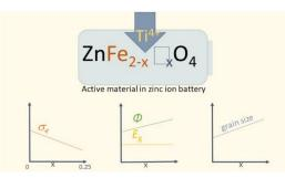
approach lies in the ability to maintain a spinel structure while exhibiting enhanced electrical properties. The doping of zinc ferrite with said tetravalent ions has been surprisingly found to create a particularly
