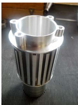
Fig. 15. Cold source prototype as developed and built for tests at the AKR-2. The cold source is a cylindrical Al vessel ( r=25 mm, l=100 mm) to condense H_2 or CH_4 gas, surrounded with a He gas cooling labyrinth. The working pressure is defined as 1.5 bar for liquid H_2 . The cold source is installed on a standard flange and can be inserted into an evacuated beam tube in the thermal moderator. 4 gas connections are used for input and output of moderator gas and He cooling gas. On the moderator surface towards the opening of the beam tube, a filter crystal can be mounted for further treatment of the spectrum.
