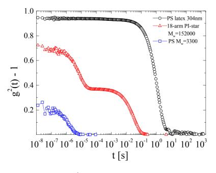
The intensity autocorrelation functions  $g^2(Q,t)$  shown here from samples with extremely different relaxation times demonstrate the large time window of dynamical light scattering.
