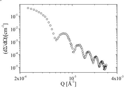
Form factor P(Q) of a hard-sphere colloid, Poly(Methylmethacrylat) in cis-Dekalin, with R=760nm,  $10^{\circ} < \Theta = 154^{\circ}$ , T=293K.
