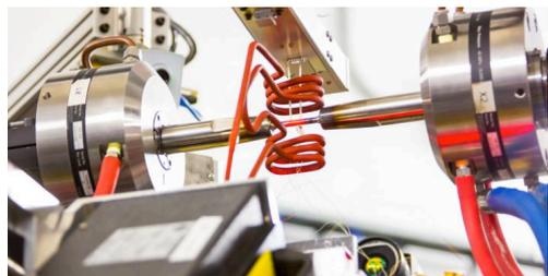
Fig. 2.3. Studying nickel-based superalloys with neutron diffraction [10]
