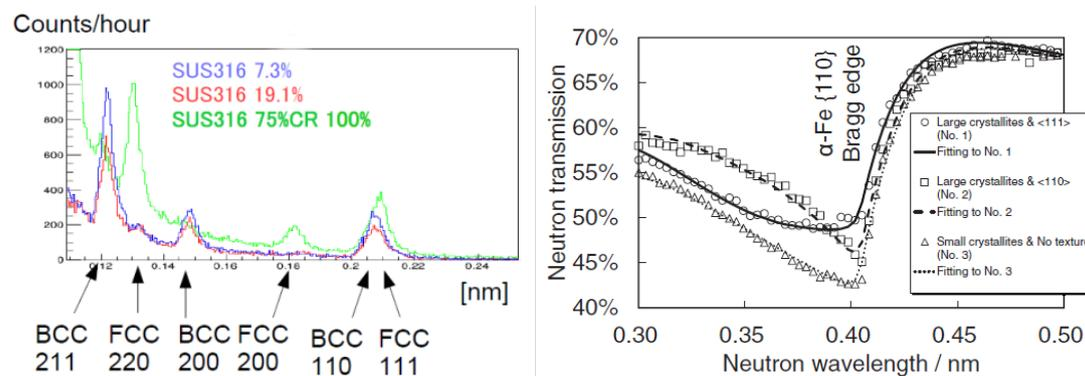
Figure A11: (left) Powder diffraction patterns on steel samples providing the austenite – martensite ratios<sup>73</sup>. (right) Bragg-edge transmission spectra measured at HUNS, and the profile fitting curves obtained by RITS.<sup>72</sup>
