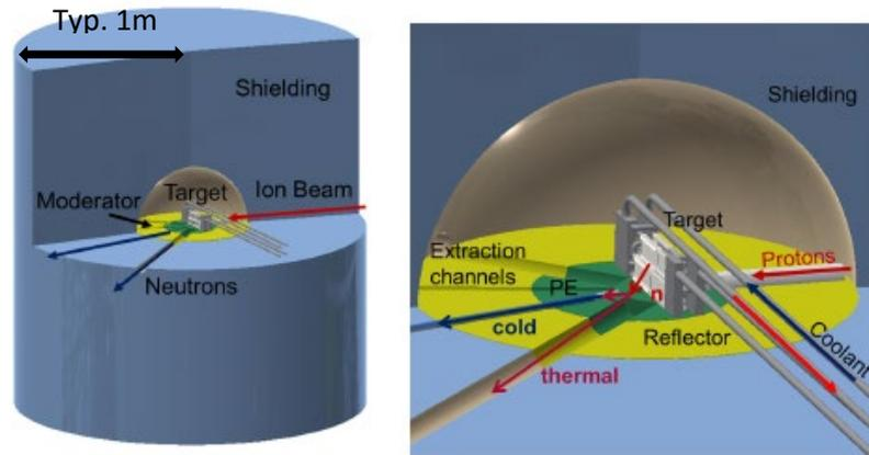
Figure 4: Sketch of target / moderator / reflector unit for CANS
