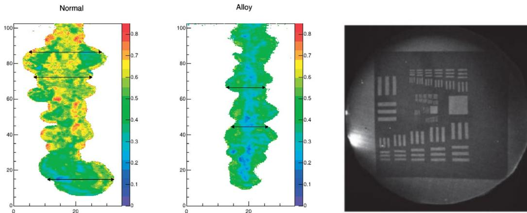
Figure A13: (left) Radiography of corroded steel plates and humidity up-take as a function of time. Pixel Size  $0.8 \times 0.8 \text{ mm}^2$ ; Measured at RANS; 5 minutes exposure time;  $E_p = 7 \text{ MeV}$ ;  $I_{av} = 15 \mu\text{A}$ ;  $P = 100 \text{ W}$ <sup>76</sup>. (right) MCP image of a USAF-1951 Gd-mask measured with the beam line of CPHS at 3MeV.
