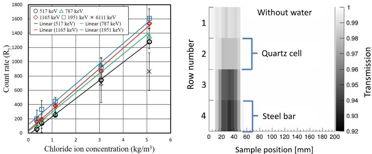
Figure A14: (left) Quantification of the chlorine content in concrete by PGA measured at RANS<sup>77</sup>. (right) Observation of water in concrete using fast neutrons<sup>78</sup>.
