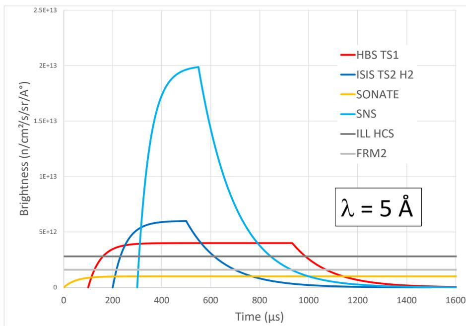
Figure A5. Single-pulse peak brightness as a function of time at a wavelength of 5 Å at HBS TS1, ISIS TS2, SNS, and brightness of ILL and FRMII cold sources. The SONATE pulse width of 2 ms is proposed to be very close to the ESS pulse structure. The starting points of the pulses have been shifted for clarity.
