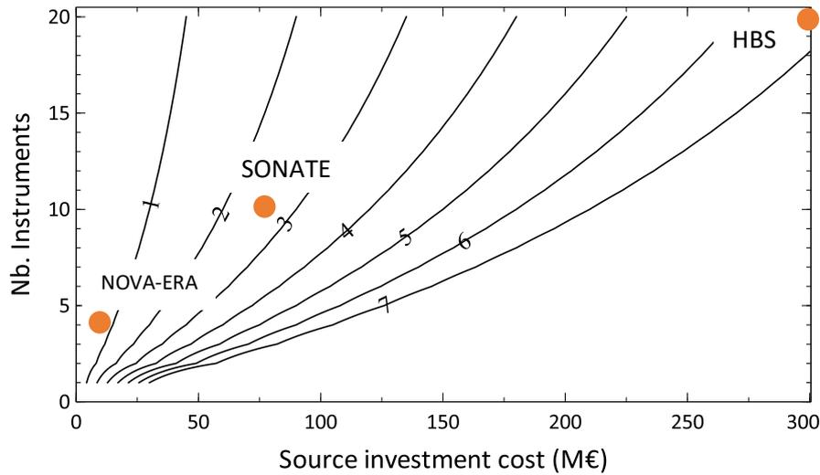
Figure 5: Dependency of the cost of an instrument-day in k€ as a function of the initial investment and the number of instruments attached to the source. The initial investment scales with the proton beam power of the source (see Fig. 3).
