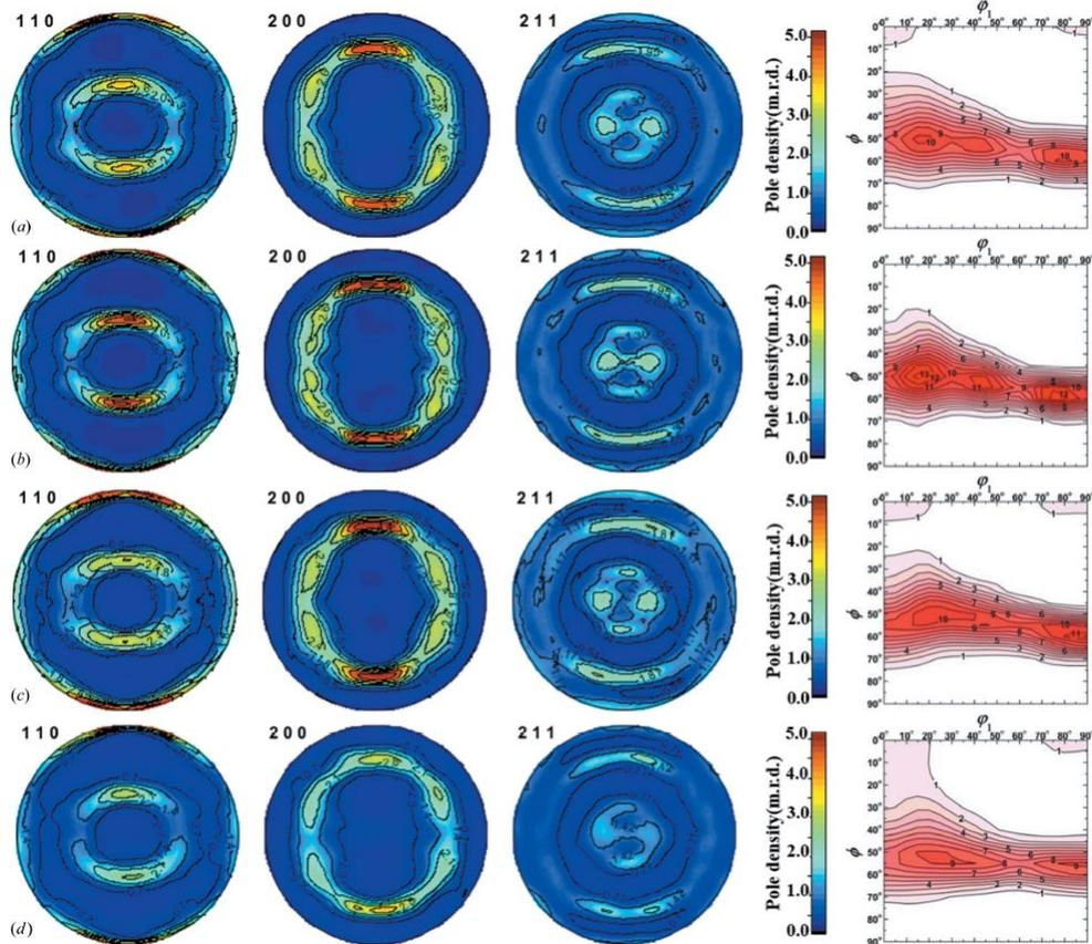
Figure A12: Example of measurements of pole figures<sup>74</sup>. (a) - (b) On RANS, with 2 different assumptions on the modelling parameters ("unequal d-range" and "equal d-range"); (c) Measurement on TAKUMI @ JPARC; (d) Measurement on HIPPO @ LANSCE.
