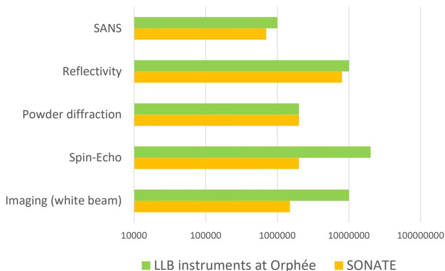
Figure A8: Comparison of the performances of different neutron scattering instruments in terms of neutron flux ( $n/cm^2/s$ ) at the sample position for LLB instruments around Orphée (green) and equivalent instruments around SONATE (yellow).
