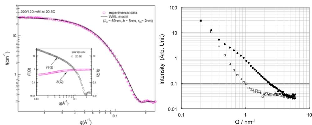
Figure A10: (left) SANS data. CTAB (200mM) micelles with 120 mM NaCl. Measured at LENS@13MeV; 20mA; 20Hz, 600 $\mu$ s;  $I_{ov} = 0.24$ mA;  $P = 3$ kW (Das et al, Langmuir 2014). (right) SANS in steel samples with (filled markers) and without (open markers) nanoscopic precipitates.<sup>72</sup>
