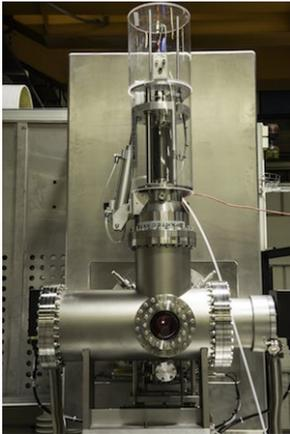
Figure A1: The ESS ion source
