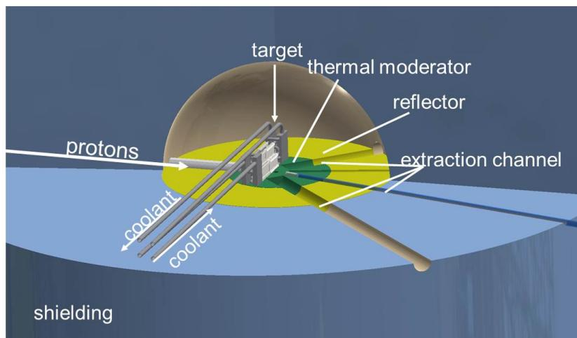
Figure A4: A possible target-moderator-reflector unit on a CANS. (green) polyethylene thermal moderator, (yellow) lead reflector.
