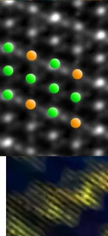
↑ Electron microscopes make tiny details visible. The colours in the top image show the different directions of the magnetic field in a 20-nanometre-thin layer of polycrystalline cobalt.
