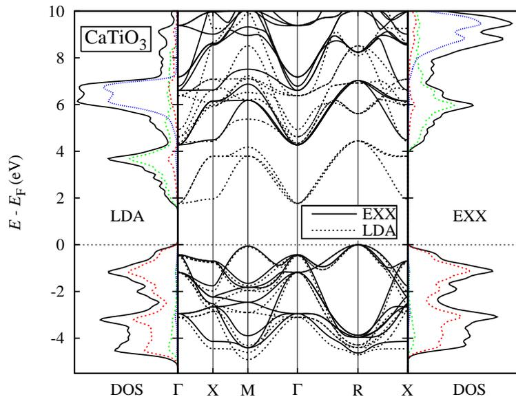
**Figure 6.15.:** LDA and EXX KS band structure and DOS for the perovskite CaTiO<sub>3</sub>. The total DOS (in units of states/eV) is shown in black, whereas the partial DOS of O 2*p*, Ti 3*d*, and Ca 3*d* is drawn in red, green, and blue.
