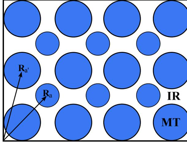
**Figure 4.1.:** Division of space into muffin-tin (MT) spheres and the interstitial region (IR). Each atomic nucleus lies in a center  $\mathbf{R}_a$  of a MT sphere of radius  $S_a$ . The radii of the spheres are chosen such that the spheres do not overlap.
