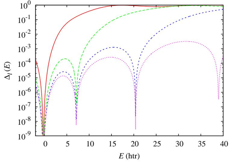
**Figure 4.3.:** Representation error  $\Delta_l(E)$  for the case of diamond and for  $l = 0$  as a function of the energy and the number of local orbitals added to the LAPW basis set. The red curve corresponds to an LAPW basis without any local orbitals, whereas for the green, blue, and magenta curves we consecutively add one local orbital more with energy parameters according to Eq. (4.18).
