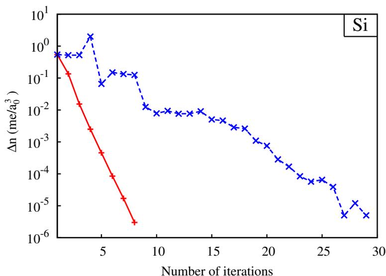
**Figure 5.3.:** Convergence behavior of the electron density for Si: the change in the density  $\Delta n$  is shown as a function of the self-consistent-field cycles. The red solid and blue dashed curves correspond to calculations with and without the nested density convergence scheme (see text).
