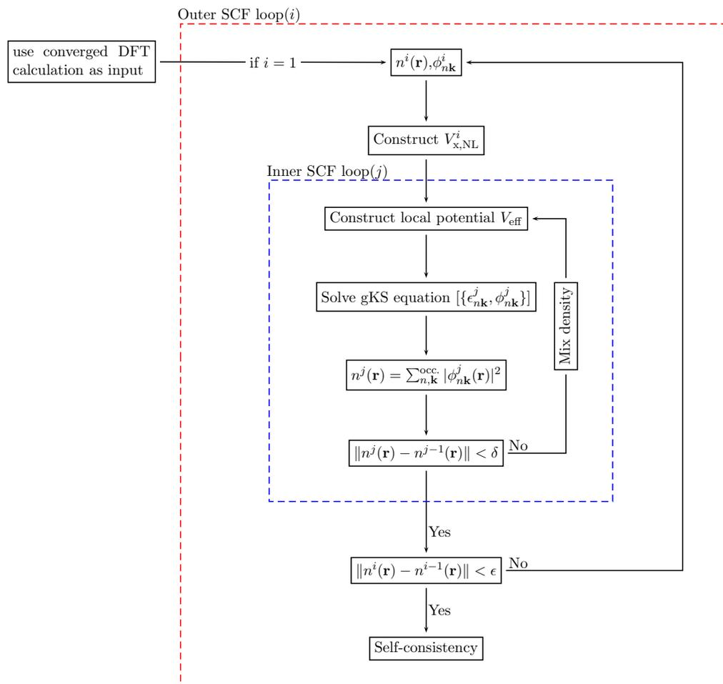
**Figure 5.4.:** Schematic illustration of the nested SCF cycle for hybrid functional calculations.
