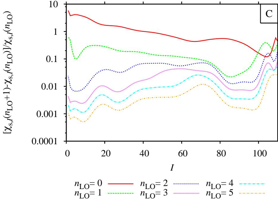
**Figure 6.5.:** Convergence of the eigenvalues of the density response function  $\chi_s$  for diamond with respect to the number of local orbitals added to the LAPW basis.  $n_{LO}$  denotes the number of local orbitals added in each  $lm$  channel from  $l = 0, \dots, 5$  to the conventional LAPW basis. The eigenvalues  $\chi_{s,I}$  are ordered according to their absolute values along the  $x$  axis. The  $y$  axis shows the relative change of the eigenvalue.
