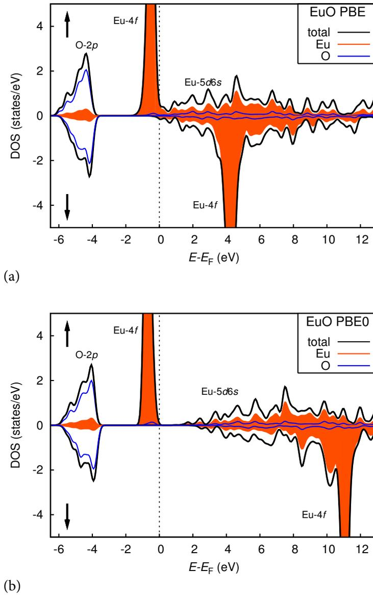
**Figure 5.9.:** Density of states (DOS) of ferromagnetic EuO for (a) the PBE and (b) the PBE0 functional. While the total DOS is shown in black, the partial DOS of Eu and O is drawn in red and blue, respectively.
