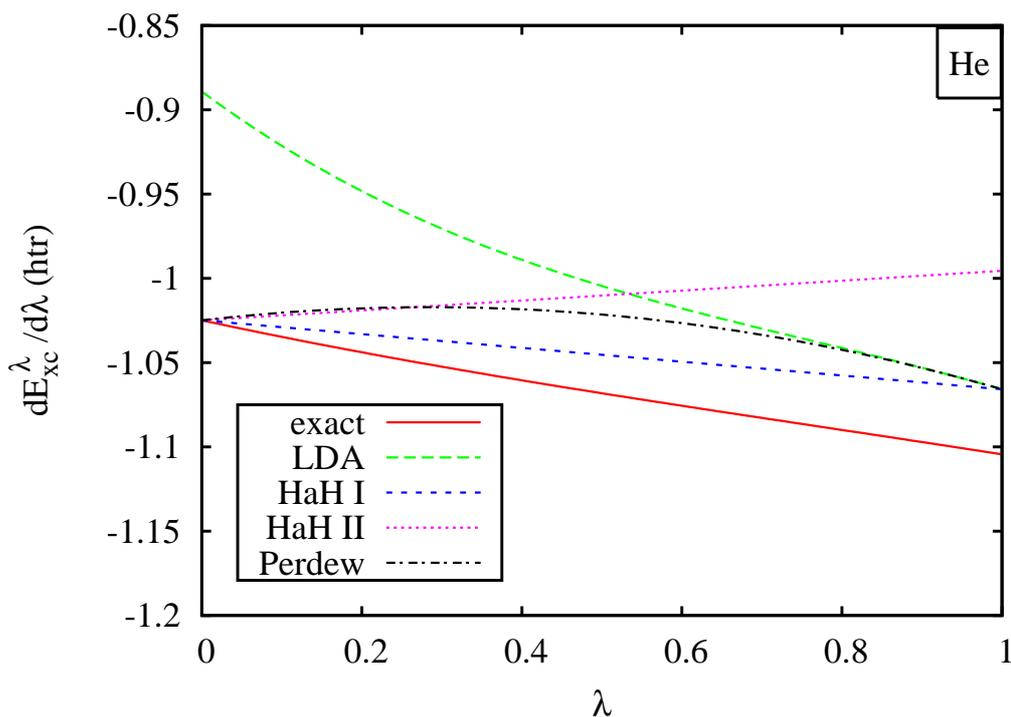
**Figure 3.2.:** The exact coupling-constant integrand  $E_{xc}^\lambda$  for the He atom is compared with the integrand in the LDA, the half-and-half hybrid according to Eq. (3.35) denoted by HaH-I, the half-and-half hybrid of Eq. (3.36) denoted by HaH-II, and finally with the hybrid proposed by Perdew *et al.* with  $n = 4$  [Eq. (3.37)]. For all three hybrids  $E_{xc}^{DF} = E_{xc}^{LDA}$  is used.
