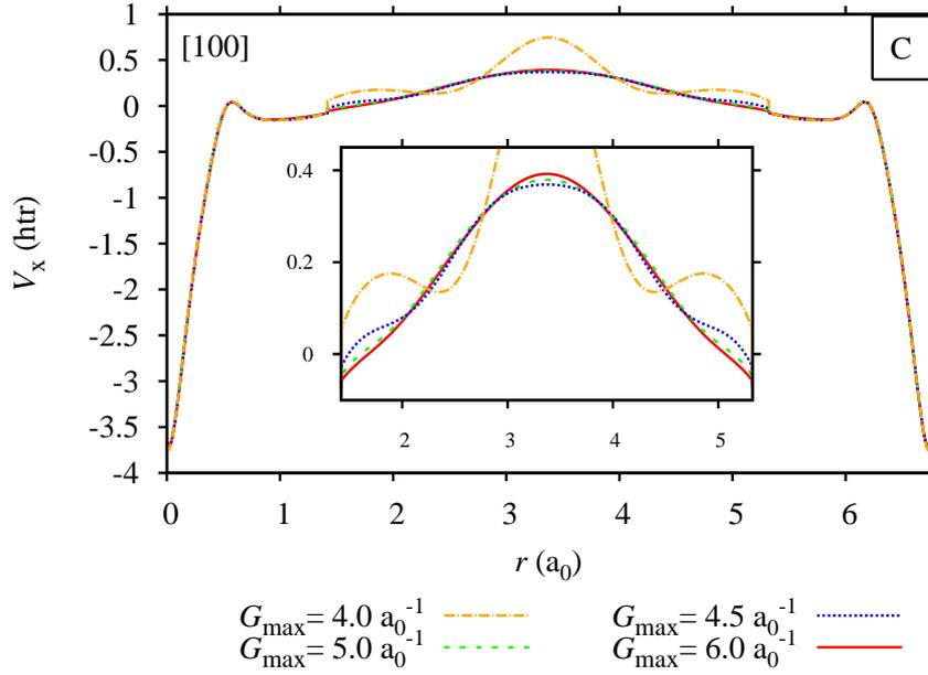
**Figure 6.4.:** The convergence of the interstitial EXX potential is demonstrated for different reciprocal cutoff radii  $G_{\max}$  of the LAPW basis on a line connecting two carbon atoms along the [100] direction. The reciprocal MPB cutoff is chosen as  $5.8 \text{ a}_0^{-1}$ .
