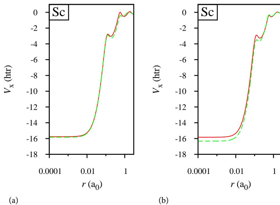
**Figure 6.13.:** (a) Comparison of  $V_x(\mathbf{r})$  around the atomic nucleus of Sc for calculations with (green dashed line,  $n_{LO} = 1$ ) and without (red solid line,  $n_{LO} = 0$ ) local orbitals. (b) Local exact exchange potential  $V_x(\mathbf{r})$  with (red solid line) and without (green dashed line) the explicit core response of the FBC.
