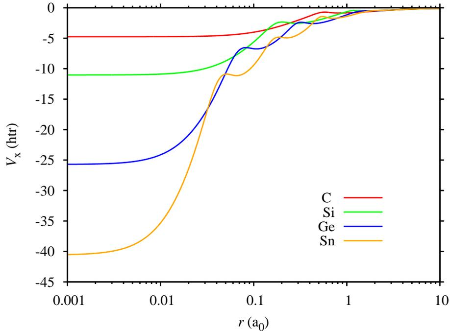
**Figure 6.1.:** Atomic EXX potentials obtained with the RELKS code for the C, Si, Ge, and Sn atom. With increasing atomic number from C ( $Z=6$ ) to Sn ( $Z=50$ ) the intershell humps move closer and closer to the atomic nuclei (at  $r = 0$ ). Simultaneously, more and more intershell humps in the EXX potential appear, one for each atomic shell.
