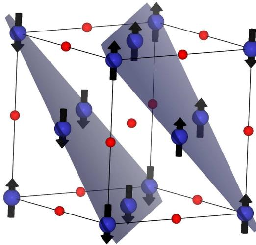
**Figure 6.18.:** Cubic unit-cell of the transition metal oxides MnO, FeO, and CoO in their antiferromagnetic order (AFM-II). The transition metal atoms with their actual spin orientation are depicted in blue, while the oxygen atoms are red.
