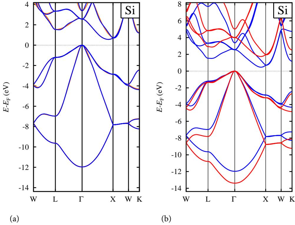
**Figure 5.6.:** (a) Comparison of routinely generated PBE (orange) and Wannier interpolated (blue) band structure for Si. (b) Comparison of PBE (blue) and the Wannier-interpolated PBE0 band structure (red) for Si.
