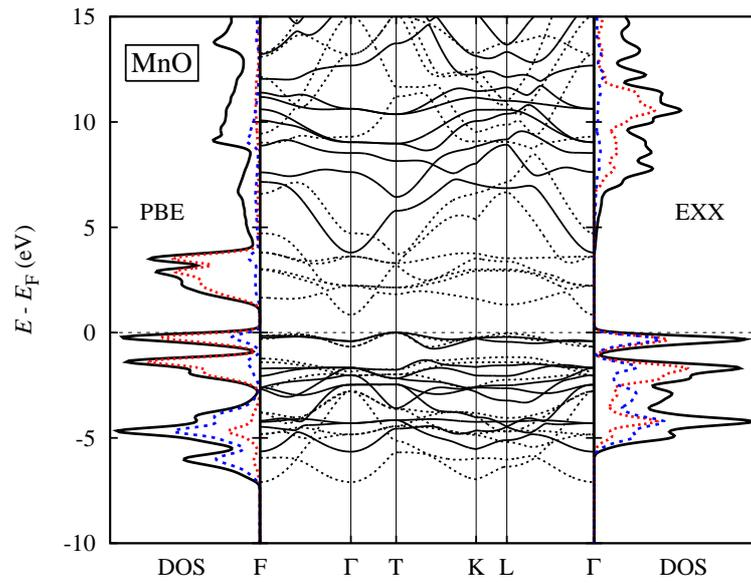
**Figure 6.19.:** PBE (dashed black lines) and EXX (solid black lines) KS band structure and DOS (in units of states/eV) for the transition-metal oxide MnO. The contribution of the TM  $d$  states to the total DOS (black line) is drawn in red. The partial DOS for the O  $2p$  states is shown in blue.
