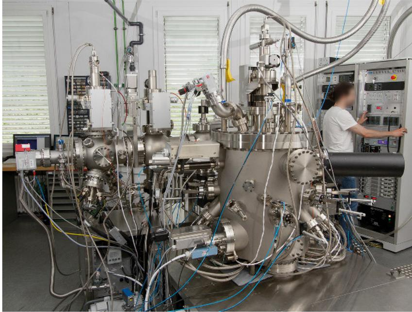
Figure 2: *The Oxide MBE used in the practical course.*
