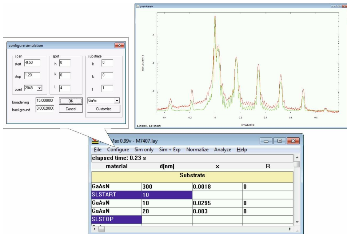
Fig 11: Screenshot of the software “MadMax” that is used to simulate XRD curves.
