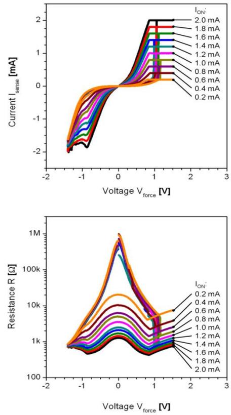
Fig. 2: Demonstration of multilevel switching of an exemplary  $HfO_2$  based test device
