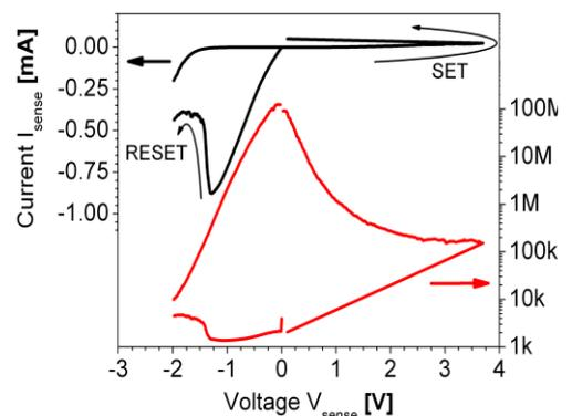
Fig. 1: Exemplary resistive switching of a HfO<sub>2</sub> based test device
