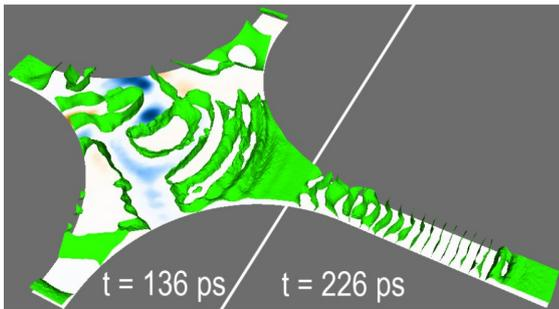
FIG. 2: Spin wave propagation in an extended branch of the sample at two different times following the field pulse maximum. The  $m_z = 0$  isosurfaces shown in green allow to visualize the wave fronts. The blue spot represents the switched core.
