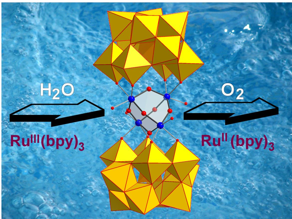
FIG. 1: Scheme of the water oxidation catalyst  $[\{\text{Ru}_4\text{O}_4(\text{OH})_2(\text{H}_2\text{O})_4\}(\gamma - \text{SiW}_{10}\text{O}_{36})_2]^{10-}$ . Ru: blue spheres, O: red spheres, tungstate units: yellow polyhedra.
