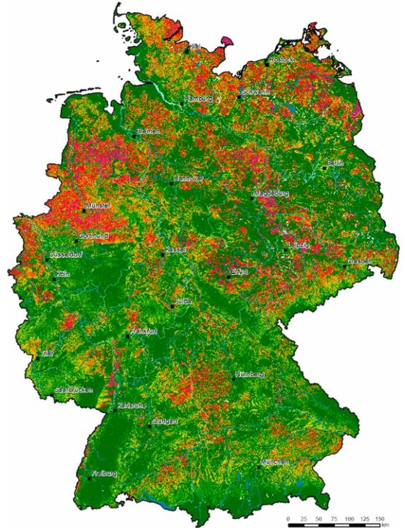
↑ Simulation of the nitrate concentration in the leachate: green signifies low nitrate concentrations and red/purple very high ones. For comparison: the EU limit for groundwater is 50 milligrams of nitrate per litre (mg NO<sub>3</sub>/L). The map shows the result of a simulation from a previous project. In RELAS, such simulations are repeated with significantly improved input data for modelling and monitoring.
